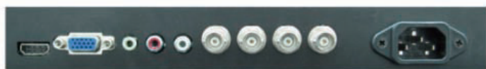
HDMI / VGA / PC Audio / RCA x 2 / BNC In x 2 / BNC Out x 2 / HDMI x 1
